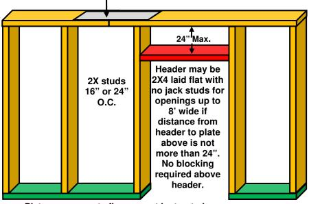
Plates on concrete floors must be treated unless there is a vapor barrier under the slab.
