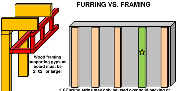
1 X Furring strips may only be used over solid backing or framing spaced not more than 24" o.c. A Furring strips placed against a concrete or masonry wall must be treated unless a vapor retarder is placed between the wall and furring strips
